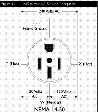
Use this receptacle to operate 120/240 Volt AC, 60 Hz, single phase loads requiring up to 7,500 watts (7.5 kW) of power. The outlet is protected by a 35 Amp push-to-reset circuit breaker.
